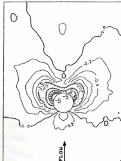
Surface pressures, high-turbulence jet, R = 4.0
