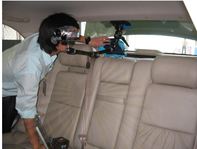
Fig.4-2(c) Attachment of a video camera
