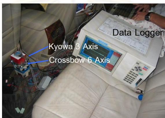
Fig.4-2(a) Position of sensors installed within a cabin
