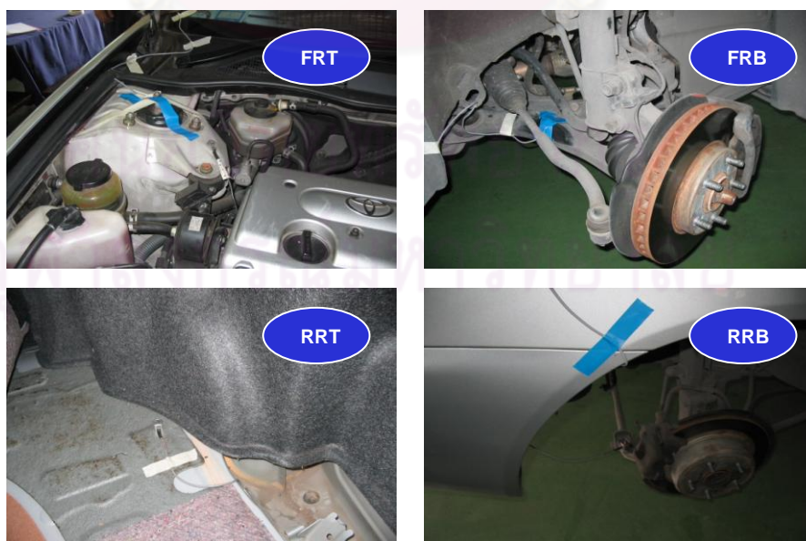
Fig.4-2(b) Positions of sensors installed outside a cabin
