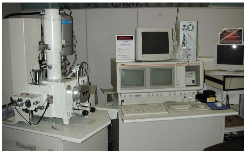
Figure 3.3 Scanning Electron Microscope (SEM)
