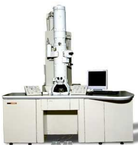
Figure 3.5 Transmission Electron Microscope (TEM)
