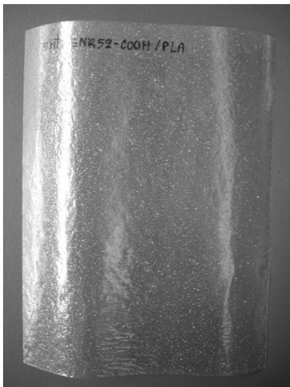
Figure F.6 Characteristic of 3 wt% ENR52-COOH/PLA film
