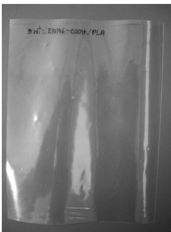
Figure F.3 Characteristic of 3 wt% ENR6-COOH/PLA film
