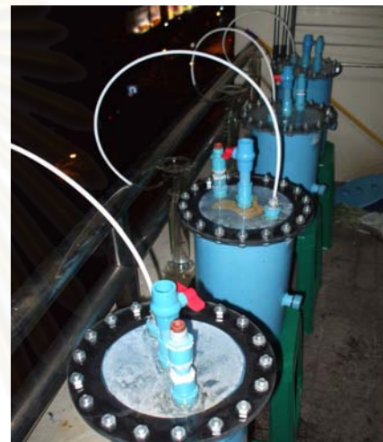
Simulated anaerobic organic waste bioreactors
