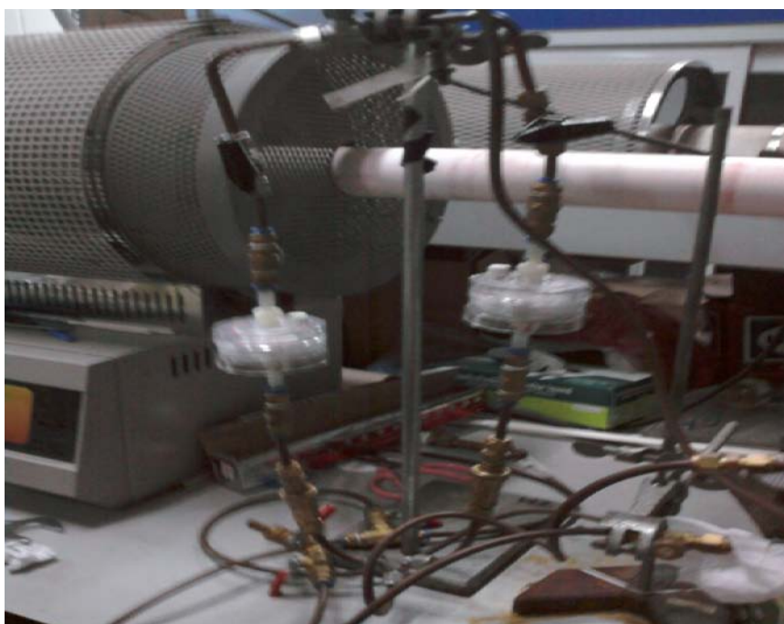
Figure 3.5 Two filter holders installed at the outlet of the collecting chamber.
