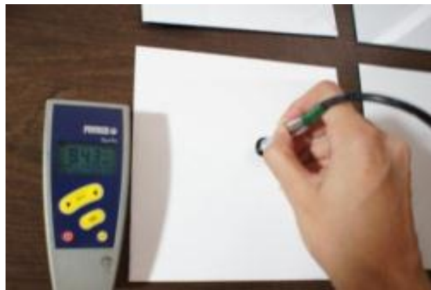
Figure 5.7 Measuring thickness of paint film
