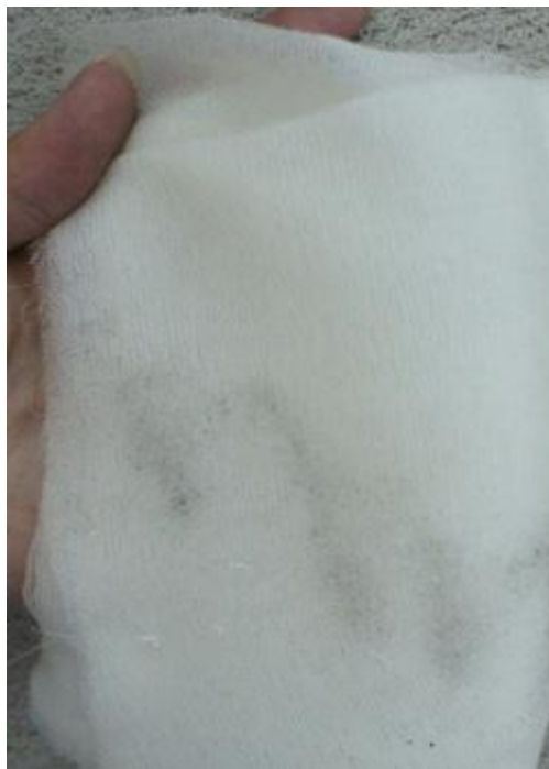
Figure 5.16 Dust on painting booth's wall
