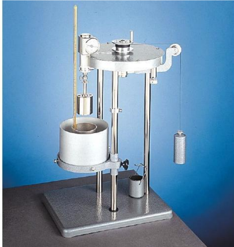
Figure 2.6 Stormer Viscometer (Thomas Scientific, 2009)
