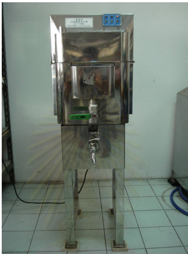
Figure B.1 Supervibration-photocatalytic reactor
