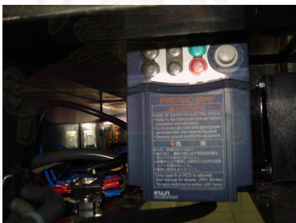
Figure B.5 Controller of vibration frequency
