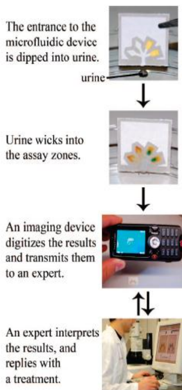
Figure 2.2 General strategy for performing inexpensive bioassays in remote locations and for exchanging the results of the tests with off-site technicians. [2]
