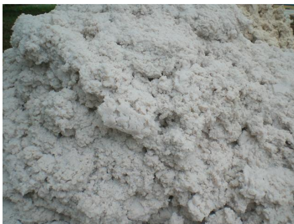
Figure1.1 The semi-sludge containing aluminium hydroxide, Al(OH) 3 .
