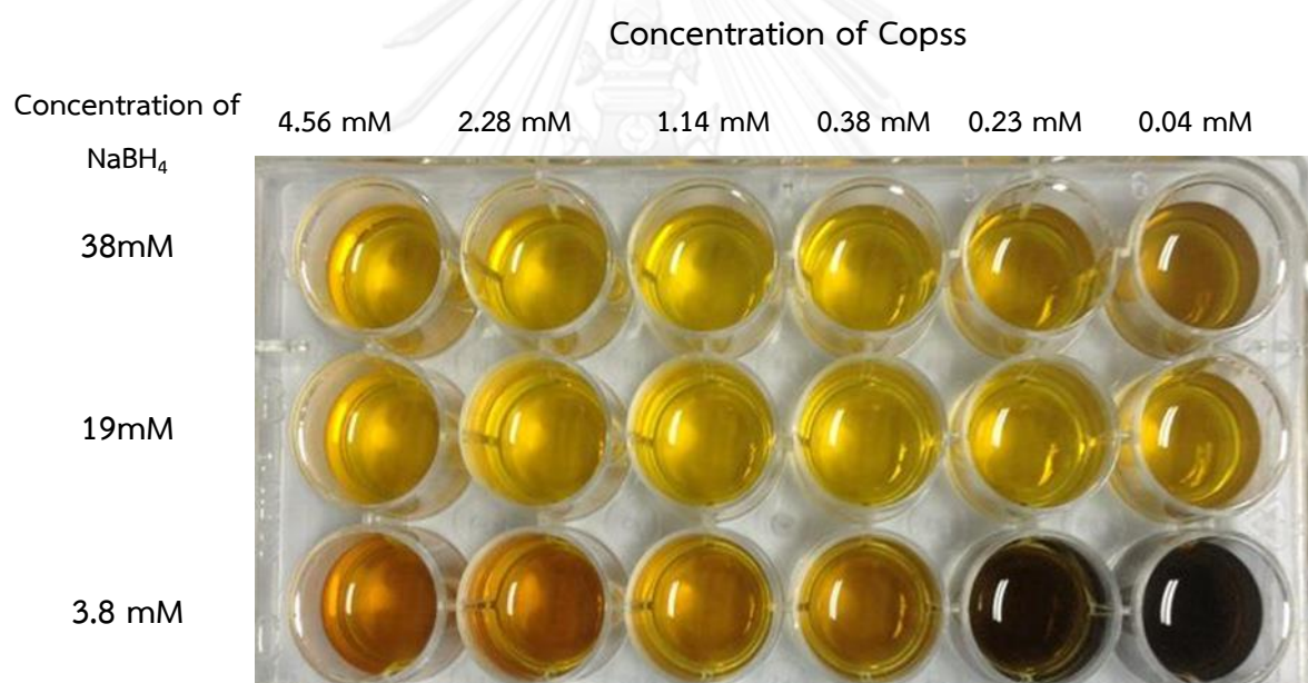
Figure 4.1 Solution of AgNPs prepared by using 3.8 mM \text{AgNO}_3 , 3.8 - 38 mM \text{NaBH}_4 and (A) 3.8 - 38 mM alginate or (B) 3.8 - 38 mM Copss. The light yellow of AgNPs indicated that the stabilized particles
