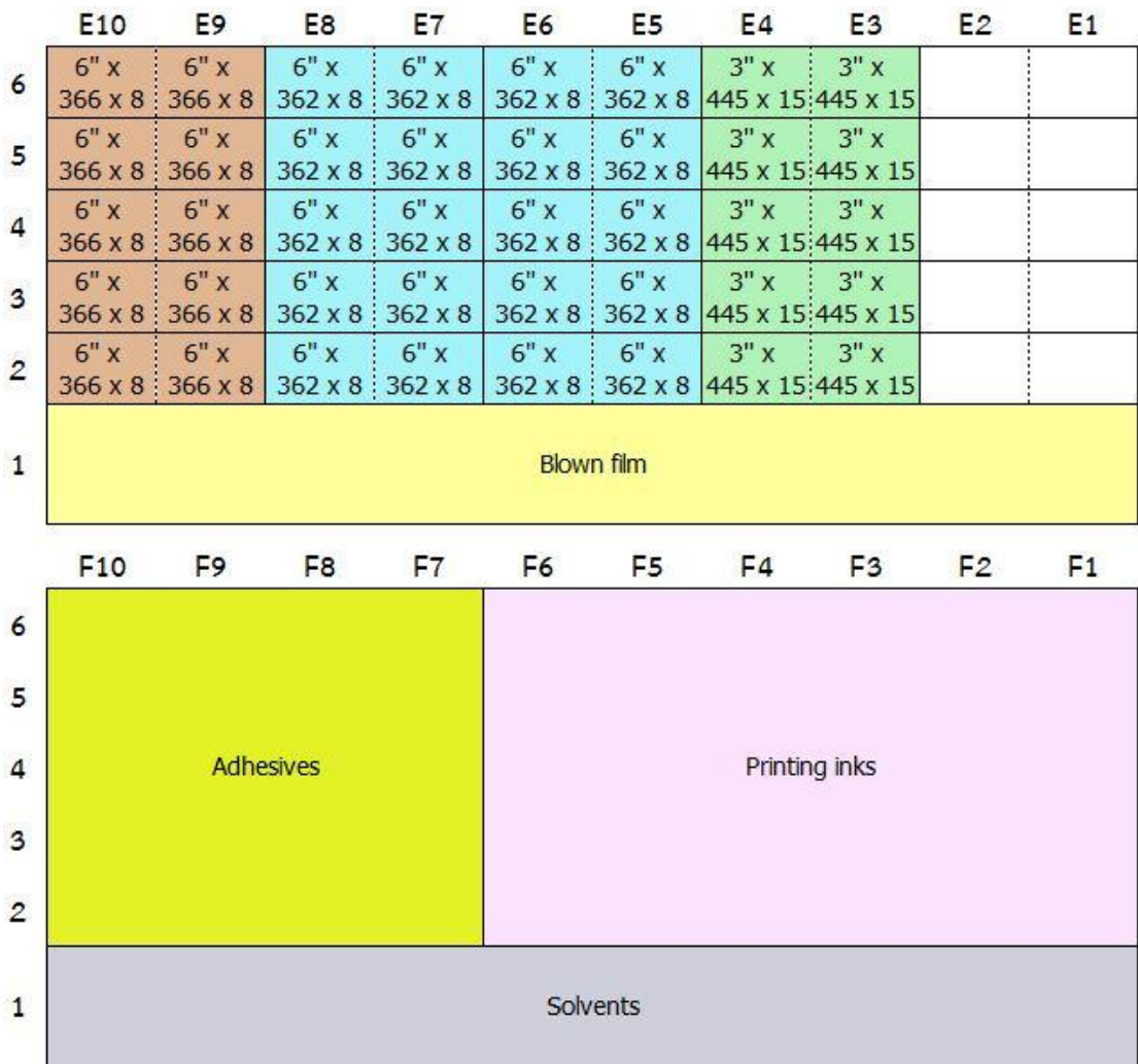
Figure 3.12: Existing warehouse slotting of paper cores, printing inks, adhesives and solvents (Zone E and F)
