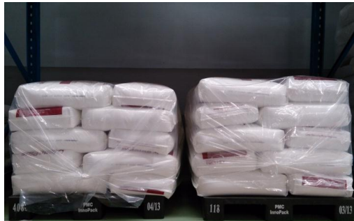
Figure 5.3: Storage condition of plastic resins and additives (I) 20 bags on pallet (II) 40 bags on pallet
