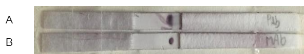
Figure 13 The positive signal of protein A/G conjugated with 40-nm commercial AuNPs on lateral flow strip, A: rabbit polyclonal anti-HPV 16 (ABIN733448) and B: mouse monoclonal anti-HPV 16 E6 were immobilized.
