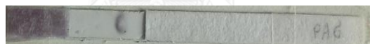
Figure 16 The positive signal of immobilized protein A/G after binding with mouse monoclonal anti-HPV 16 E6 (ab70) conjugated 40-nm commercial AuNPs on lateral flow strip.
