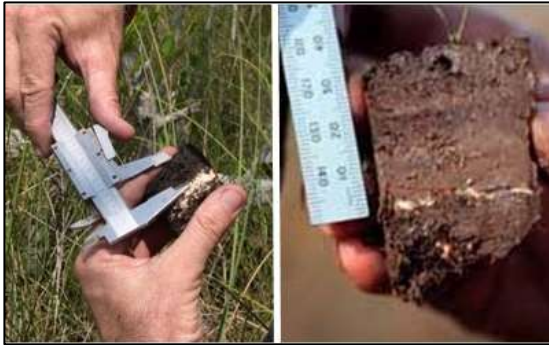
(ก) วิธี marker horizon (Southeast Ecological Science Center; 2013; Patuxent Wildlife Research Center, 2003)
