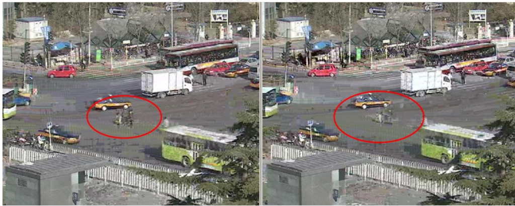
Figure 4.9 The distortion of compress video frame for Crossroad 256kbps from frame number 1485 between RM09 and Proposed method
