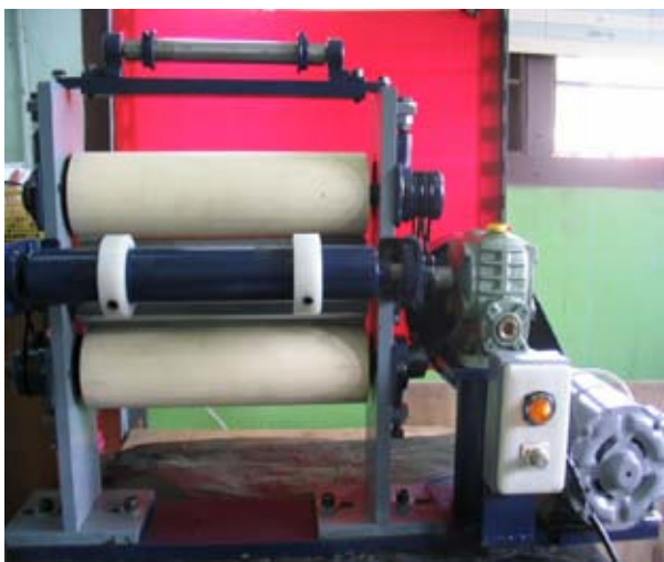
Fig. 1 A device for applying adhesive patterns
