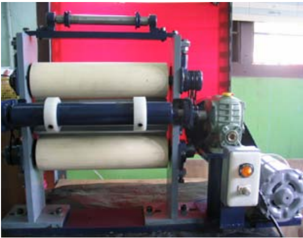
Fig. 2 A device for applying adhesive patterns
