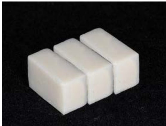
Figure 12 Fully sintered rectangular zirconium-oxide ceramic blocks (5x5x10 mm)
