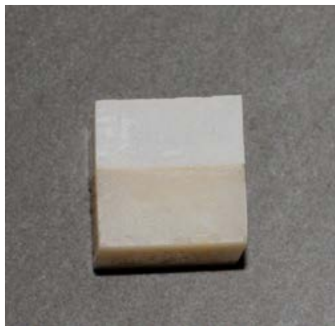
Figure 17 The zirconia-resin specimens were bonded with cement.
