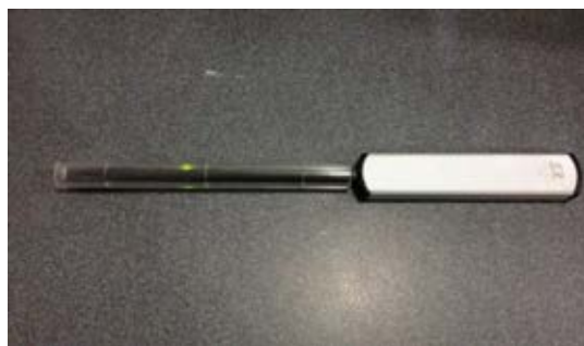
Figure 3.5 10 cm length of the pencil-type ionization Unfors Xi CT Detector
