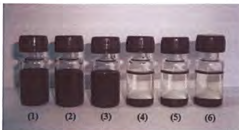
Figure 3.3 Vials (6mL) containing the CB suspension (0.15 wt/v%), in which the CB to SDS ratios were 1:0.4 (1), 1:0.8 (2) and 1:2 (3); samples were imaged after sonication 3 months whereas 1:5 (4), 1:10 (5) and 1:100 (6); samples were imaged after sonication 36-48 hours.
