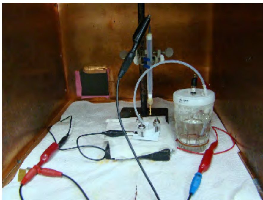
Figure 3.2 The electrochemical cell for cyclic voltammetry experiment.
