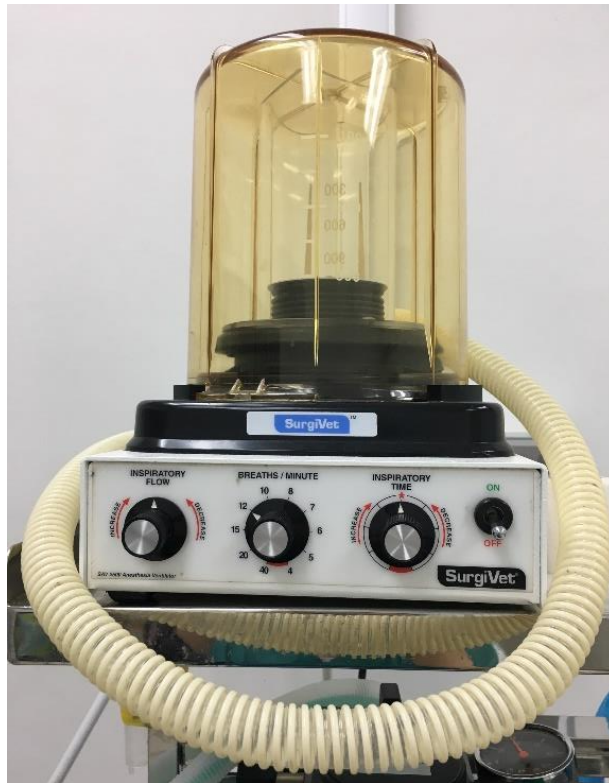
Figure 4 An anesthesia ventilator (SAV 2500 Surgivet™, Smiths Medical PM, Inc., Waukesha, WI, USA).
