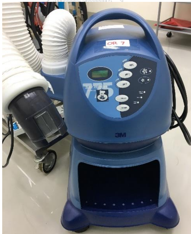
Figure 5 A warming unit (3M Bair Hugger™ Temperature Management Unit Model 775, 3M Health care, St. Paul, MN, USA).
