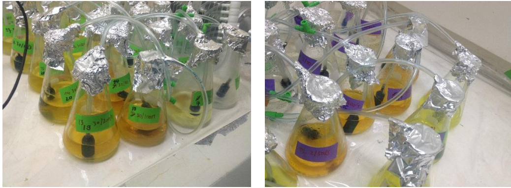
Figure 10 Tests of ammonia-oxidizing activity of nitrifying sludge under the presence of PNP
