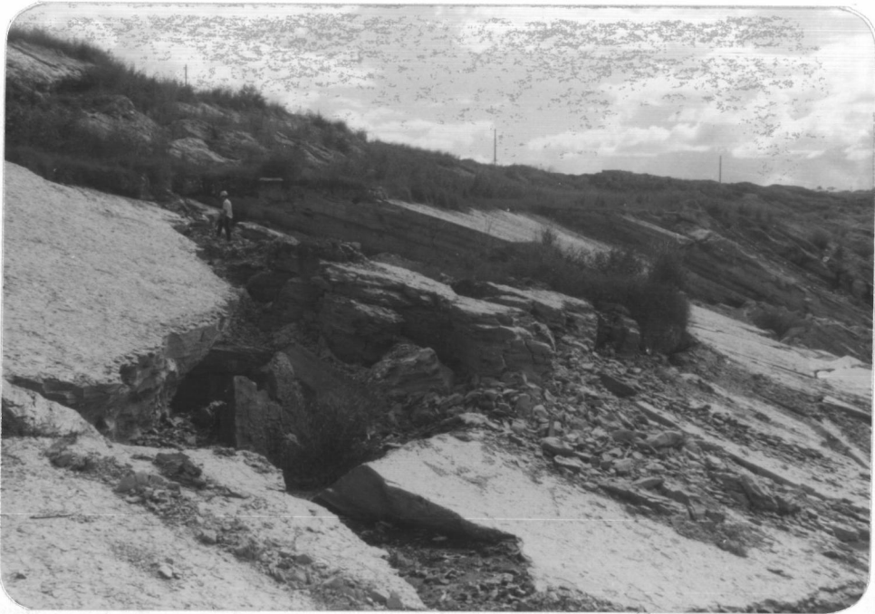
Figure 19. Planar sliding in Subarea 5.
