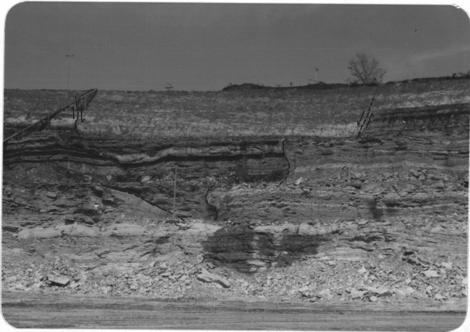
Figure 14. The northwestern flank slope of Subarea 4 showing a graben bounded by two normal fault planes.
