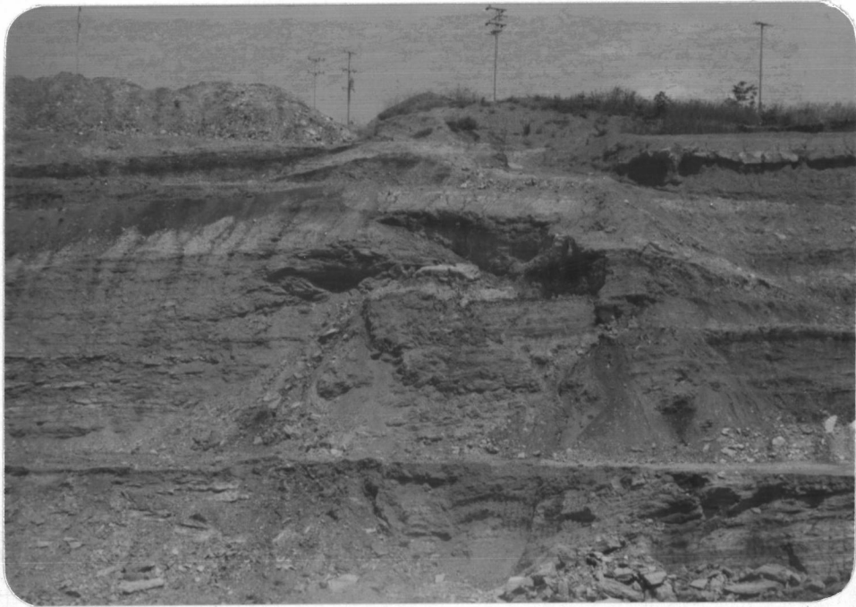
Figure 17. Enlargement of wedge failure of the northwestern flank slope (Figure 16) in March, 1981.
