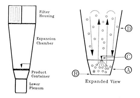
Figure 2 Top Spray Coater: (A) Product Container; (B) Air
