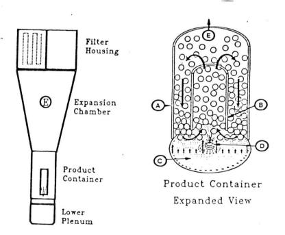
Figure 3 Wurster Bottom Spray Coater: (A) Coating Chamber;
