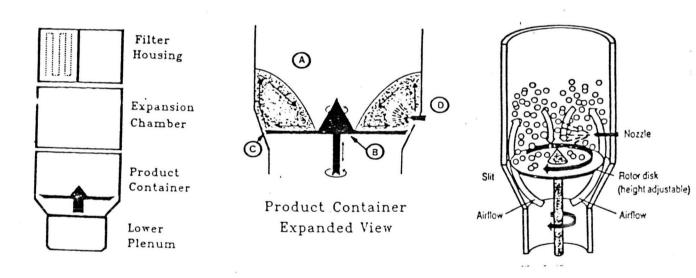
Figure 5 Rotor Tangential Spray Coater: (A) Product
