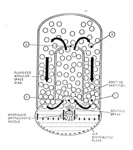
Figure 4 Diagram of the Wurster Coating Chamber.
