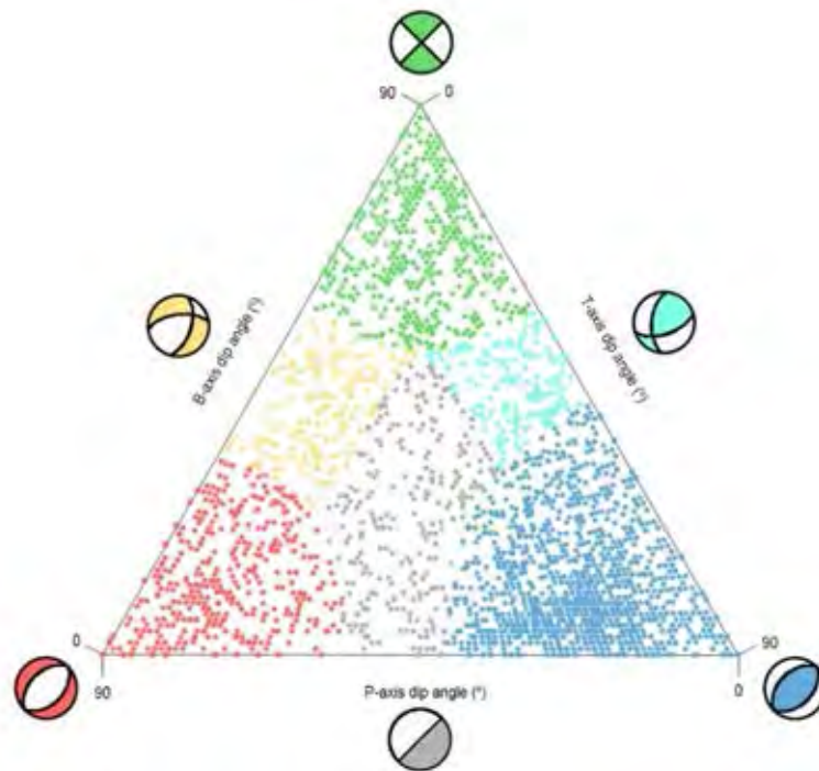
Figure 4.1. Ternary diagram showing the distribution of faulting mechanisms of all events. The classification is based on Frohlich and Anderson (1992).
