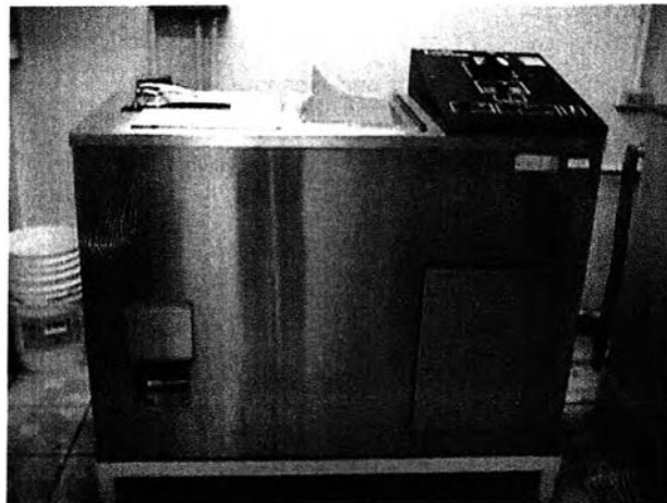
Figure 3.14 Launder-Ometer machine for colour fastness to washing
