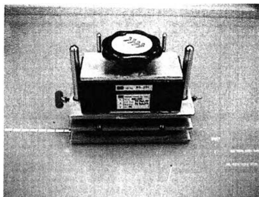
Figure 3.15 Perspiration tester machine for colour fastness to water test
