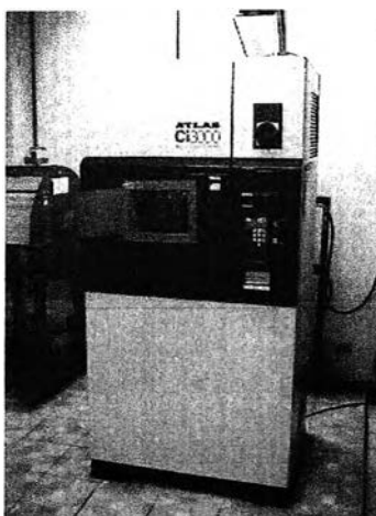
Figure 3.12 Fade-Ometer machine for colour fastness to light test
