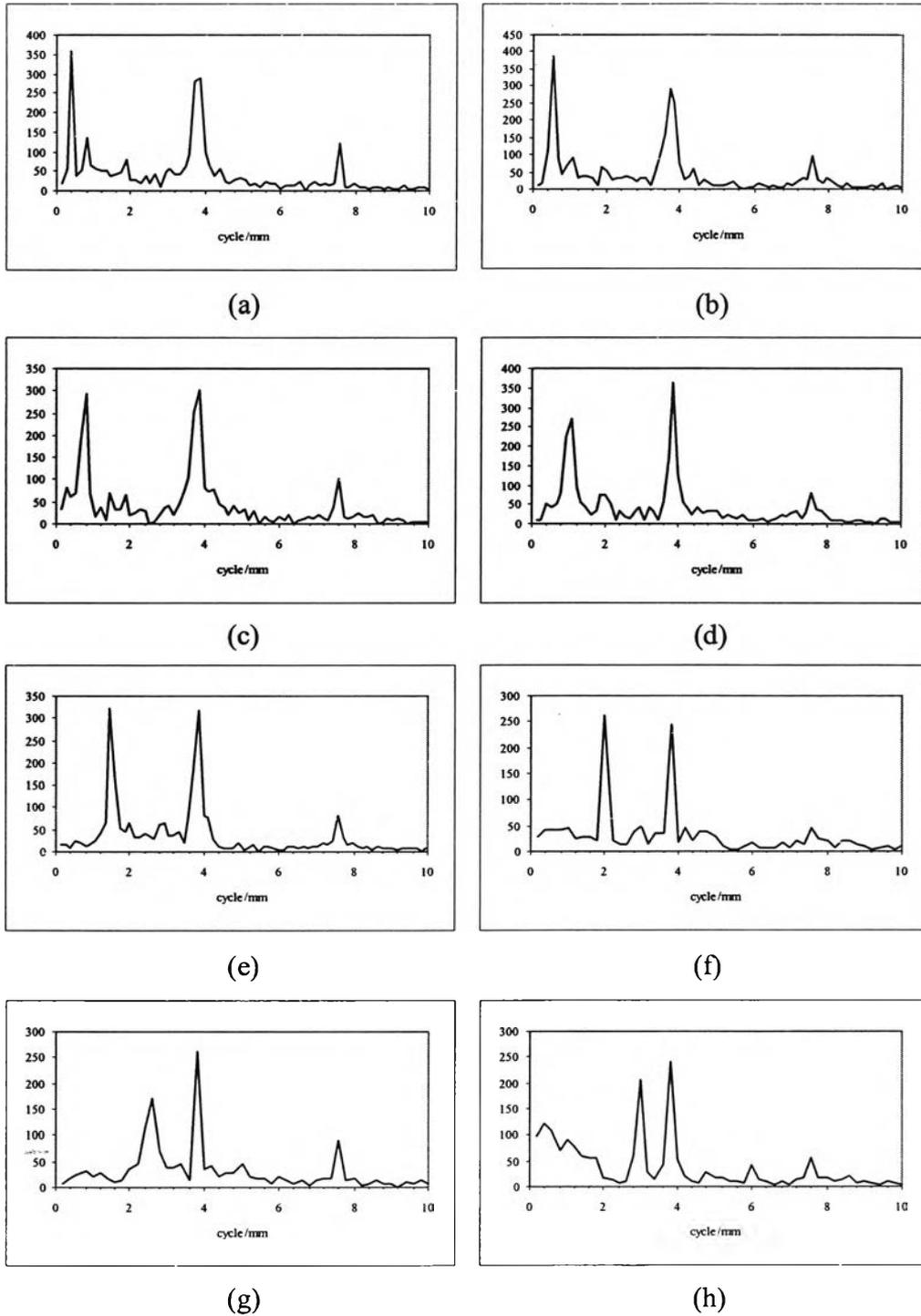
**Figure 4.11** Fourier spectrum of the test pattern on silk D at spatial frequencies (a) 0.375, (b) 0.5, (c) 0.75, (d) 1.0, (e) 1.5, (f) 2.0, (g) 2.5, (h) 3.0 cycles/mm.
