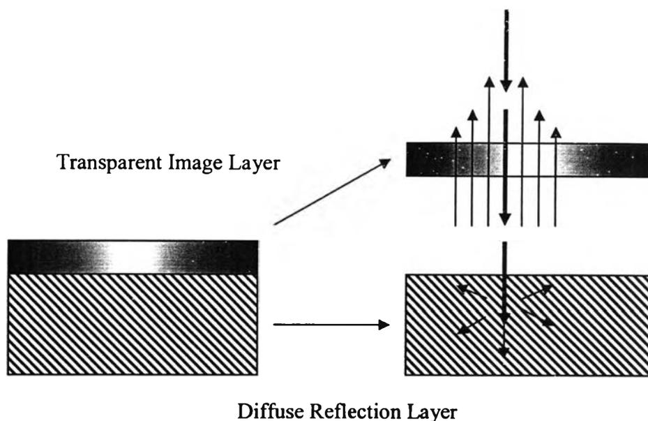
**Figure 4.18** Diagram of reflection image model
