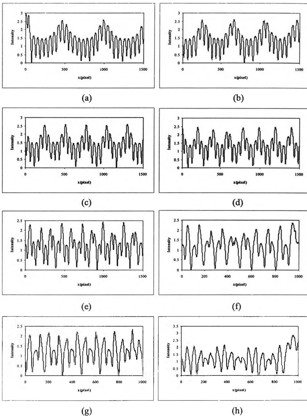
**Figure 4.6** Traces of the contacted sinusoidal test pattern for the silk fabric D by the microdensitometer at the different applied spatial frequencies of (a) 0.375, (b) 0.5, (c) 0.75, (d) 1.0, (e) 1.5, (f) 2.0, (g) 2.5, (h) 3.0 cycles/mm.
