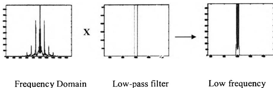
**Figure 4.13** Resulting of low-pass filter
