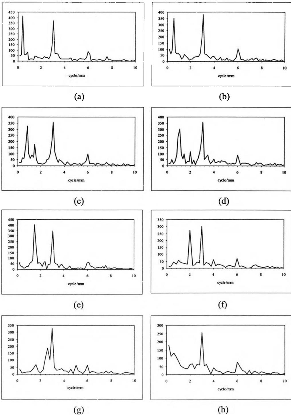
**Figure 4.10** Fourier spectrum of the test pattern on silk C at spatial frequencies (a) 0.375, (b) 0.5, (c) 0.75, (d) 1.0, (e) 1.5, (f) 2.0, (g) 2.5, (h) 3.0 cycles/mm.
