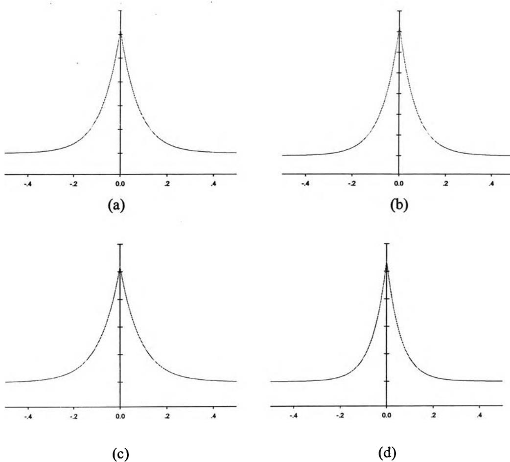
**Figure 4.17** Point Spread Function of Silk Fabrics (a) Silk A, (b) Silk B, (c) Silk C and (d) Silk D.
