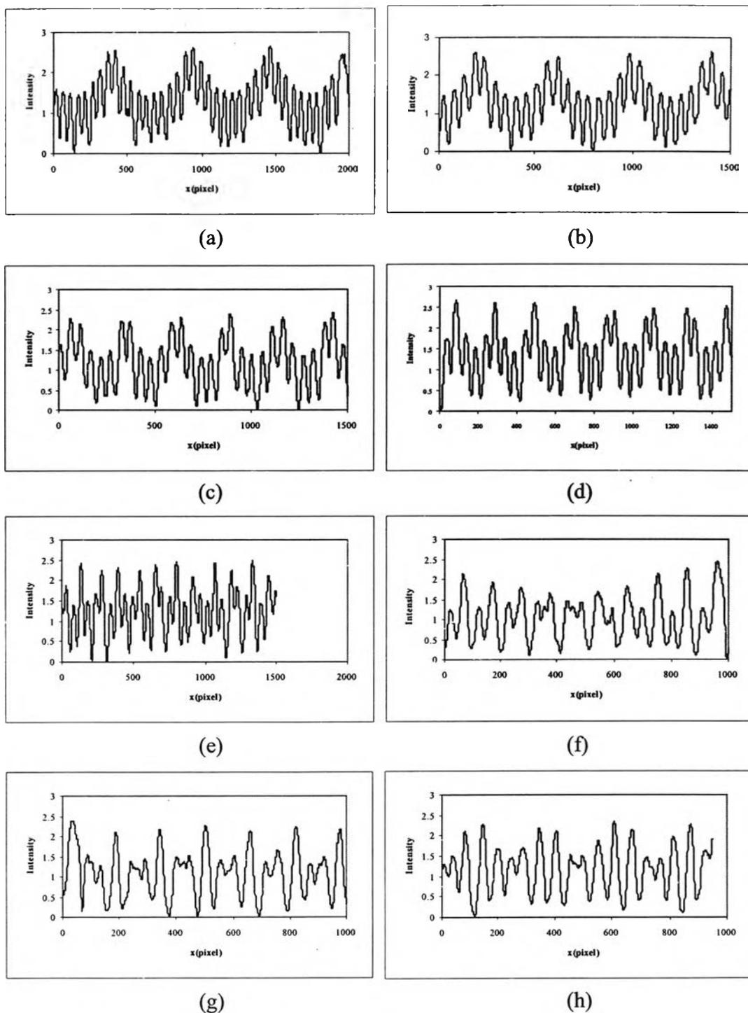
**Figure 4.3** Traces of the contacted sinusoidal test pattern for the silk fabric A by the microdensitometer at the different applied spatial frequencies of (a) 0.375, (b) 0.5, (c) 0.75, (d) 1.0, (e) 1.5, (f) 2.0, (g) 2.5, and (h) 3.0 cycles/mm.
