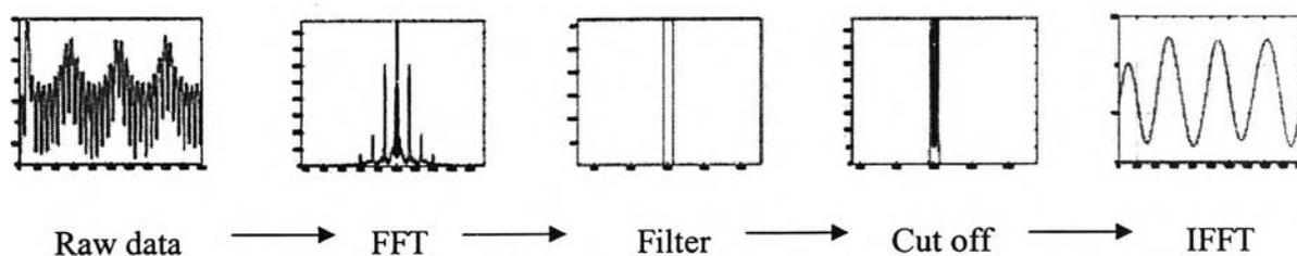
Figure 4.14 Steps of low-pass filter
