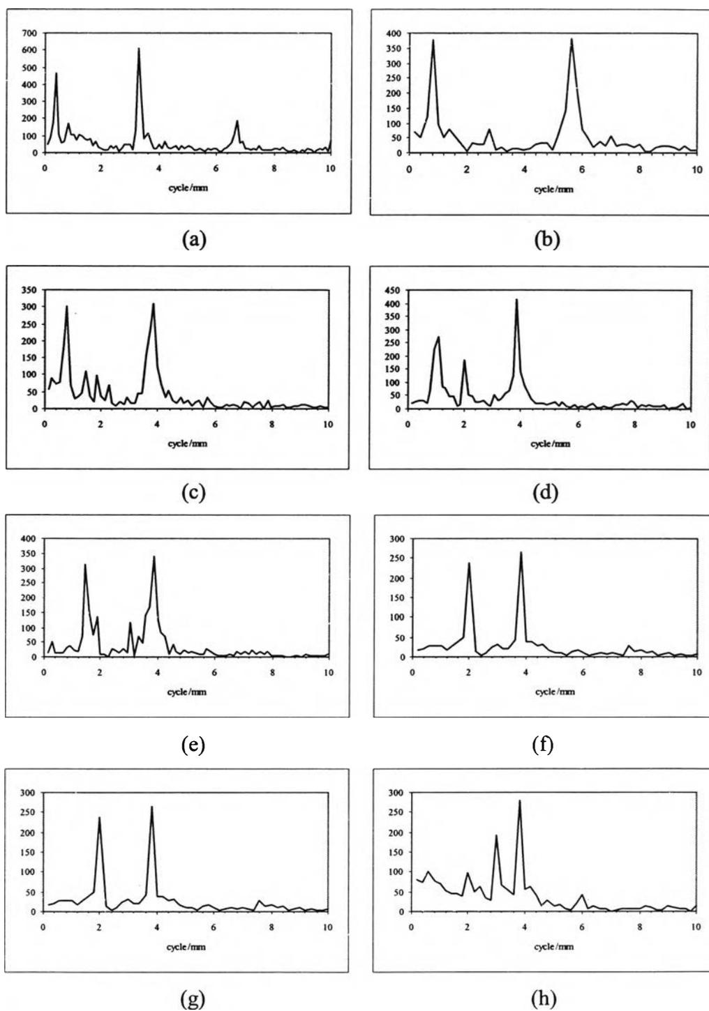
**Figure 4.8** Fourier spectrum of the test pattern on silk A at spatial frequencies (a) 0.375, (b) 0.5, (c) 0.75, (d) 1.0, (e) 1.5, (f) 2.0, (g) 2.5, (h) 3.0 cycles/mm.
