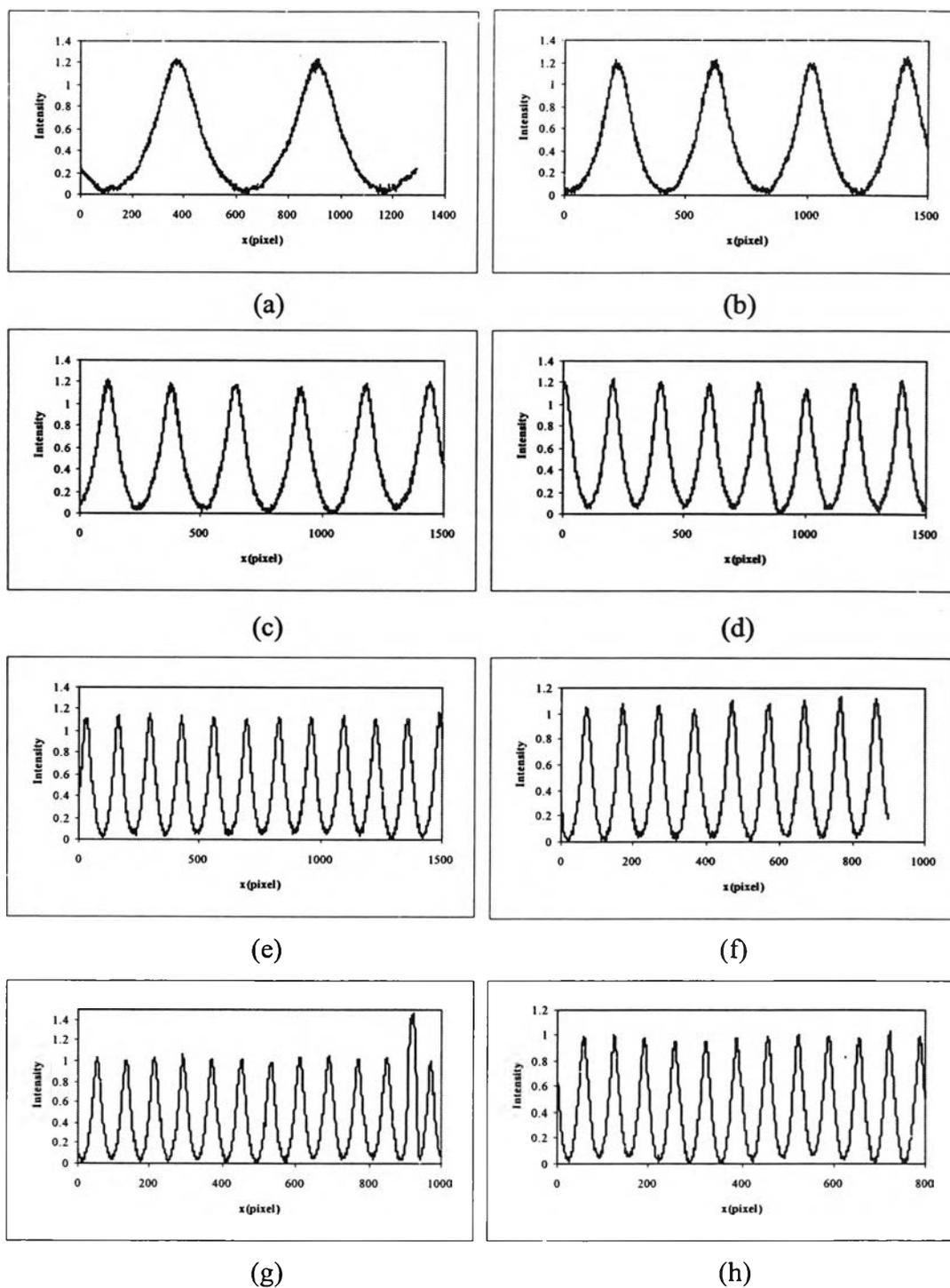
**Figure 4.7** Traces of the contacted sinusoidal test pattern for the paper by the microdensitometer at the different applied spatial frequencies of (a) 0.375, (b) 0.5, (c) 0.75, (d) 1.0, (e) 1.5, (f) 2.0, (g) 2.5, (h) 3.0 cycles/mm.
