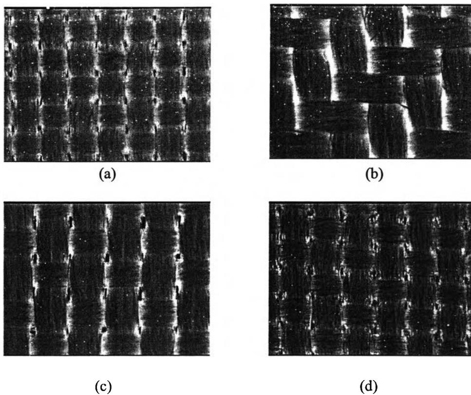
**Figure 4.2** Structural images of the silk fabrics (a) silk type A, (b) silk type B, (c) silk type C, and (d) silk type D
