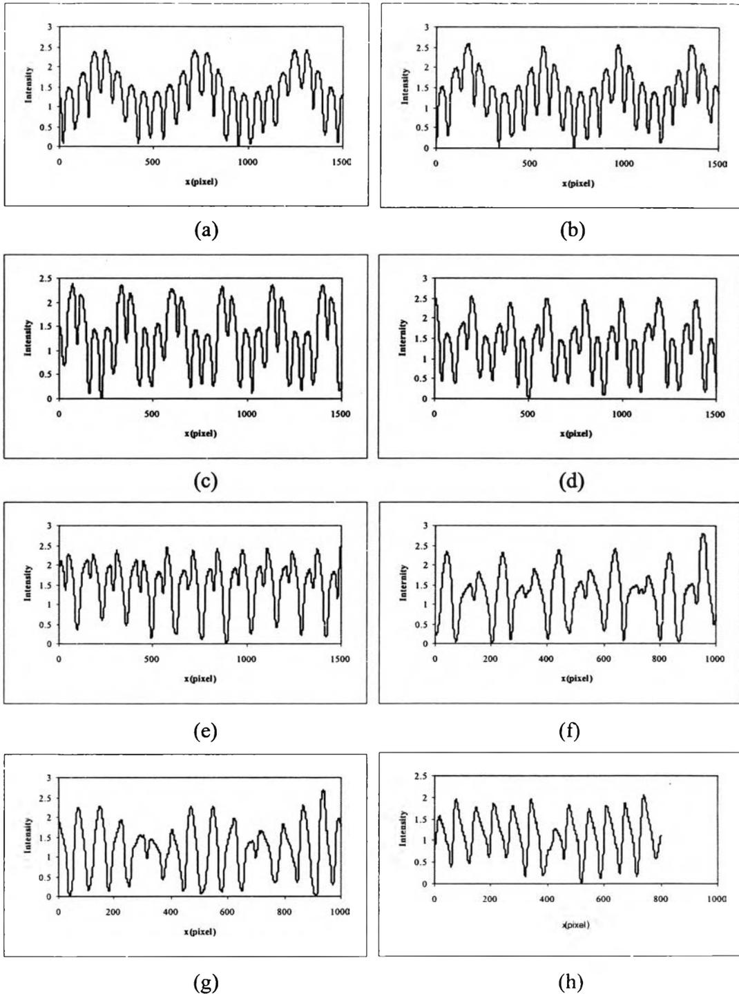
**Figure 4.5** Traces of the contacted sinusoidal test pattern for the silk fabric C by the microdensitometer at the different applied spatial frequencies of (a) 0.375, (b) 0.5, (c) 0.75, (d) 1.0, (e) 1.5, (f) 2.0, (g) 2.5, (h) 3.0 cycles/mm.
