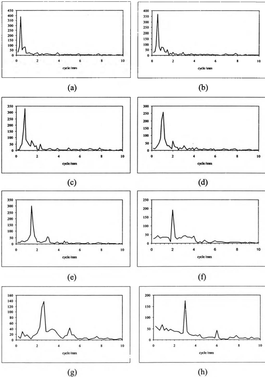
**Figure 4.9** Fourier spectrum of the test pattern on silk B at spatial frequencies (a) 0.375, (b) 0.5, (c) 0.75, (d) 1.0, (e) 1.5, (f) 2.0, (g) 2.5, (h) 3.0 cycles/mm.
