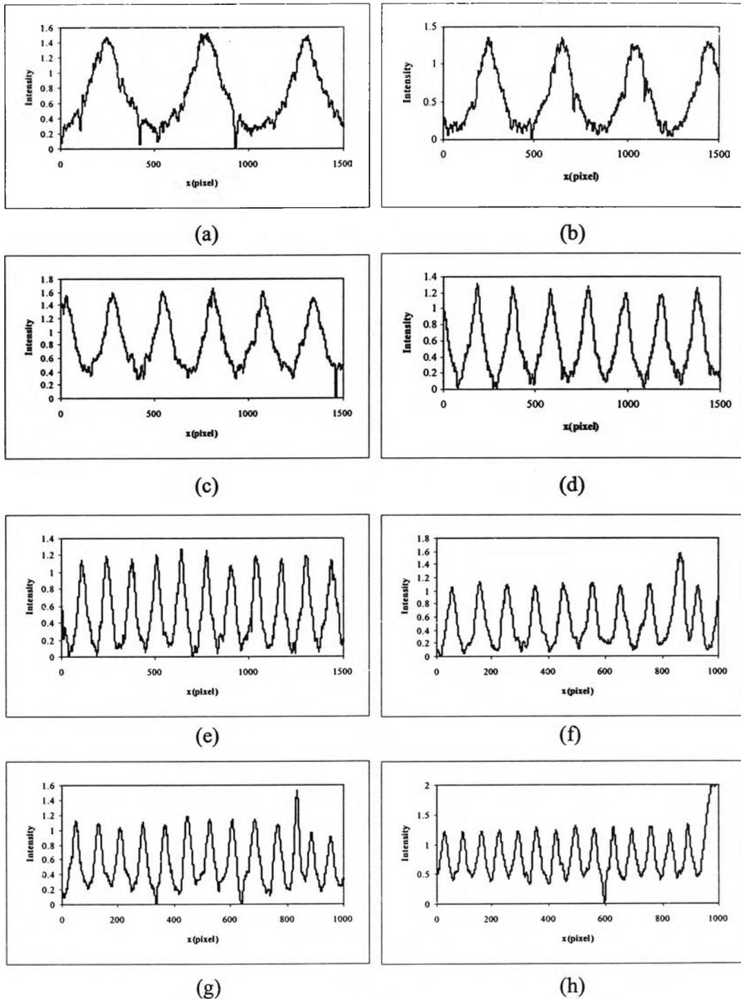
**Figure 4.4** Traces of the contacted sinusoidal test pattern for the silk fabric B by the microdensitometer at the different applied spatial frequencies of (a) 0.375, (b) 0.5, (c) 0.75, (d) 1.0, (e) 1.5, (f) 2.0, (g) 2.5, (h) 3.0 cycles/mm.
