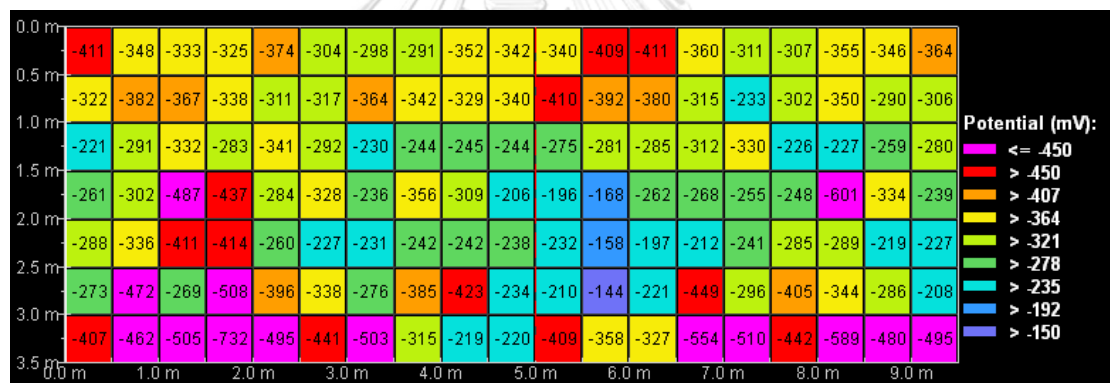
Figure 57 Example of half-cell potential result
