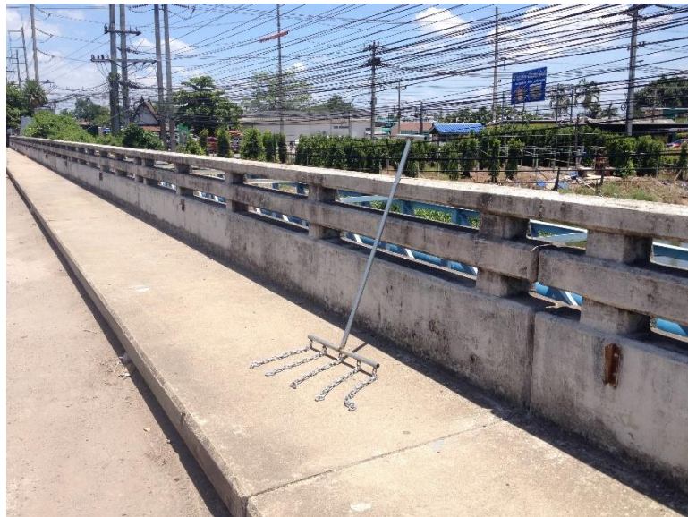
Figure 6 Chain drag equipment based on ASTM D4580
