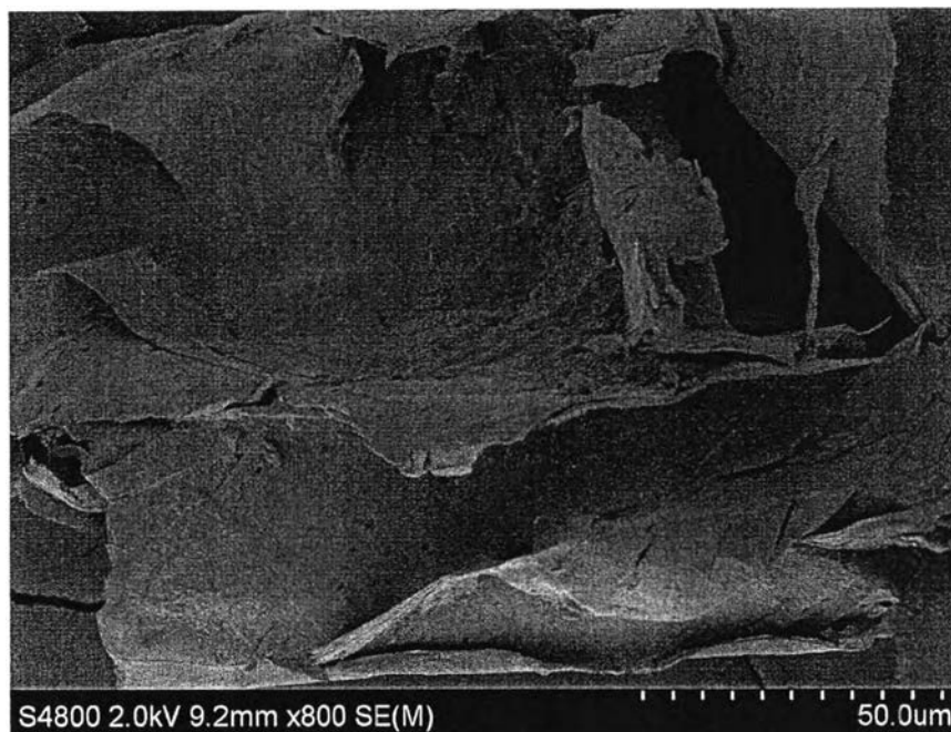
Figure G7 Scanning electron micrographs of the bagasse surface after hydrolysis of > 80 mesh bagasse with 300 U cellulase enzyme loading at 37 °C.
