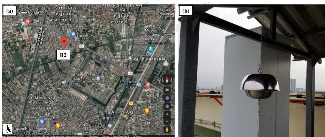
Figure 14 : Location of sampling points (B2), Khwaeng Thung Song Hong, Bangkok (b) PAS installation at the sampling site
