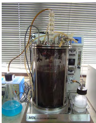
Fig. 3.3 Endoglucanase and \beta -glucosidase production in 10 liter batch reactor
