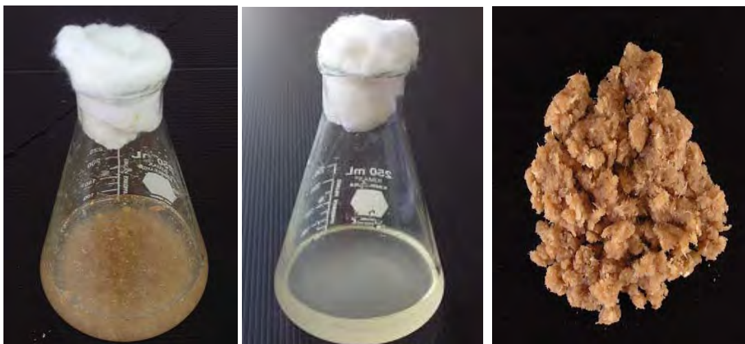
Fig. 4.1 Saccharified cassava waste (A), cassava waste hydrolysate (B) and cassava fiber (C).
