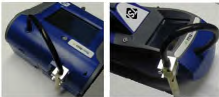
Figure 2-8: Installing Dorr-Oliver Cyclone
