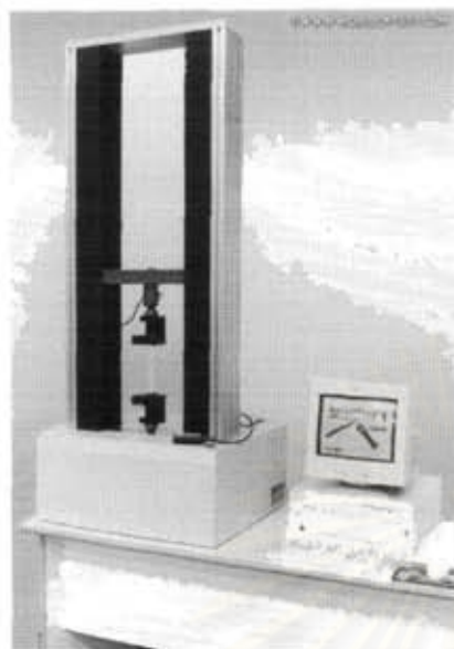
Tensile testing machine- Instron Corporation Series IX Automated Materials Testing System 6.05 Model 1011 (USA)
