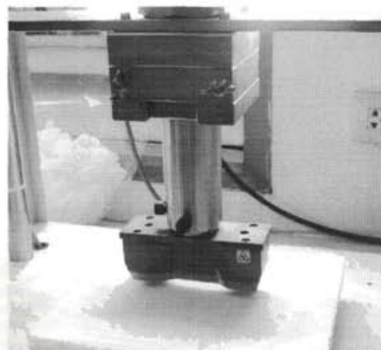
Compressed air sample cutter- Model SDAP-100-N Intro Enterprise Co., Ltd. (USA)
