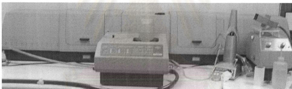
Figure A3.3 Laser particle size analyzer : Mastersizer S long bed Ver. 2.11 Serial Number : 32734 – 89
