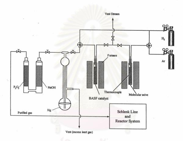
Figure 4.1.1 Inert gas supply system
