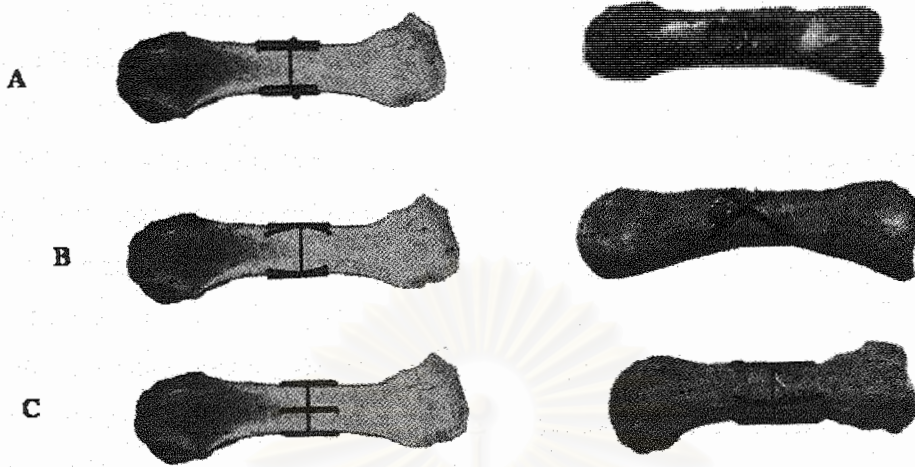
Figure 1. Antero-posterior and lateral views of experimental group A: Four knots, two parallel lateral intraosseous wire loop fixation; B: Four knots, two crossed lateral intraosseous wire loop fixation and C: Control group, 90-90 wire loops fixation.
