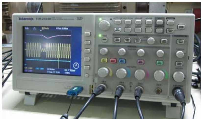
Figure 3.6 Observation of voltage sag using oscilloscope.
