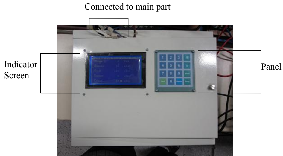
Figure 3.5 Control part of voltage sag generator.
