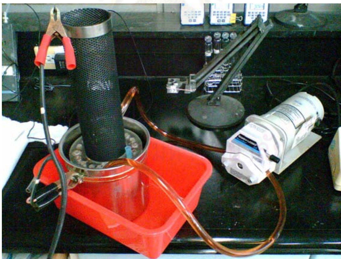
Figure A.4 electro-Fenton reactor setup for explosive wastewater degradation.
