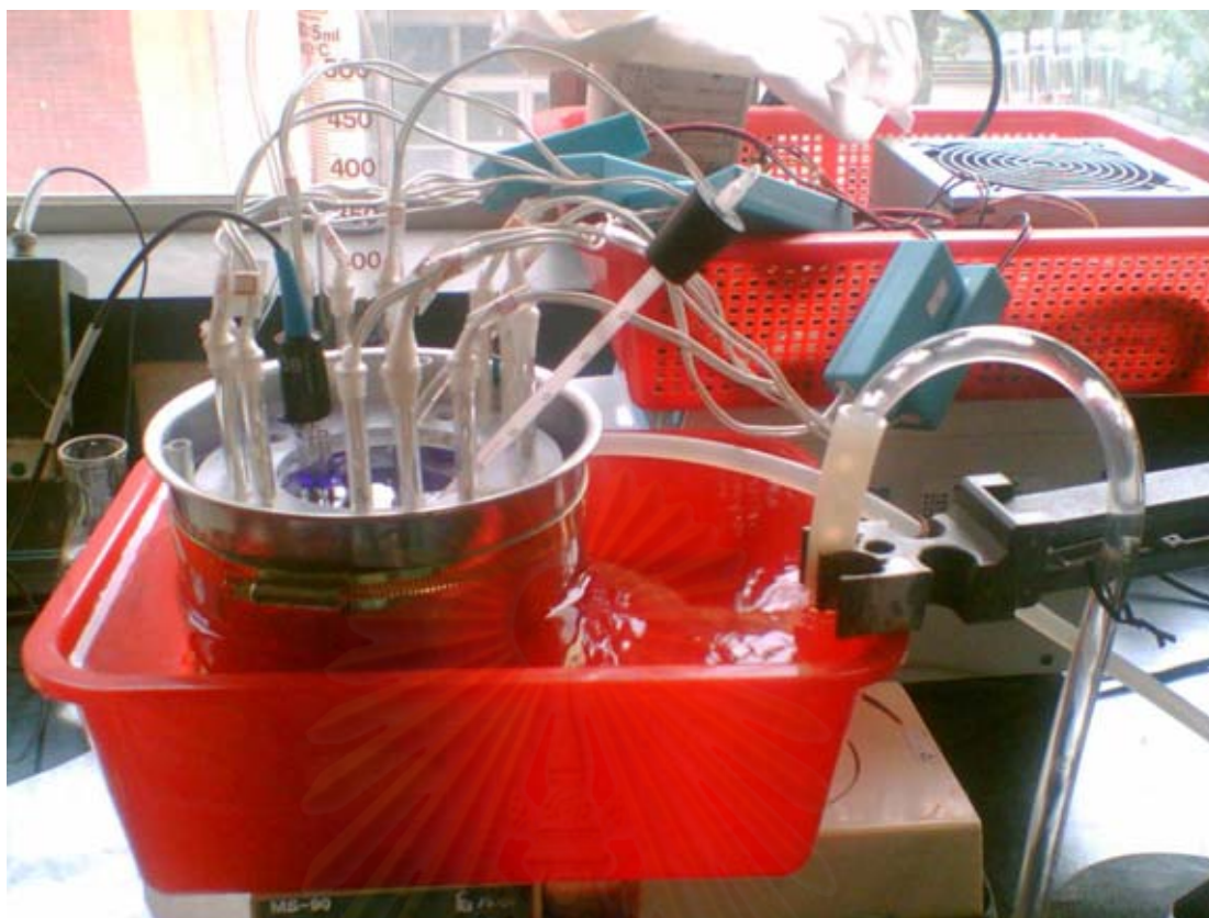
Figure A.3 photo-Fenton reactor setup for explosive wastewater degradation.
