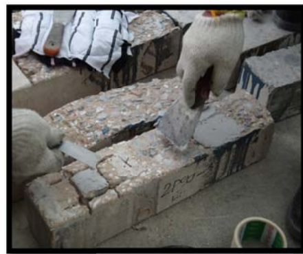
(b) Chipping off concrete surface to size of 5x5 cm.
