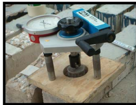
(d) Measuring surface tensile strength by tensile loading device
