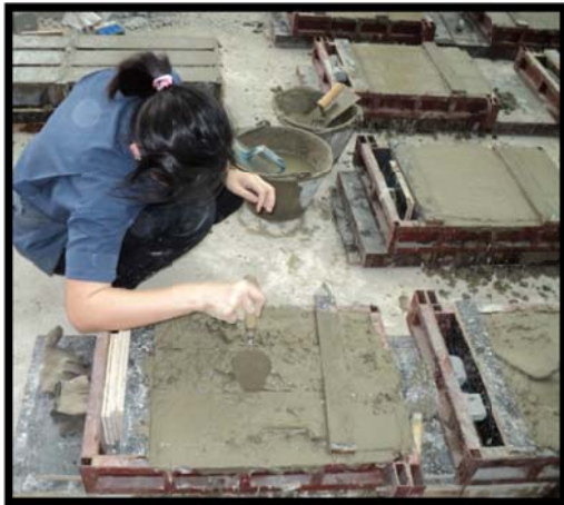
Figure 20 Molding Concrete Specimen
