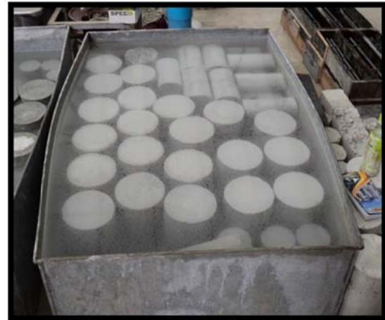
Figure 21 Curing Concrete specimens
