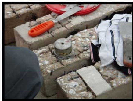
(c) Attached the steel disk by epoxy
