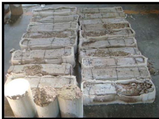
Figure 24 Burnt specimens at exposure time of 90 mins
