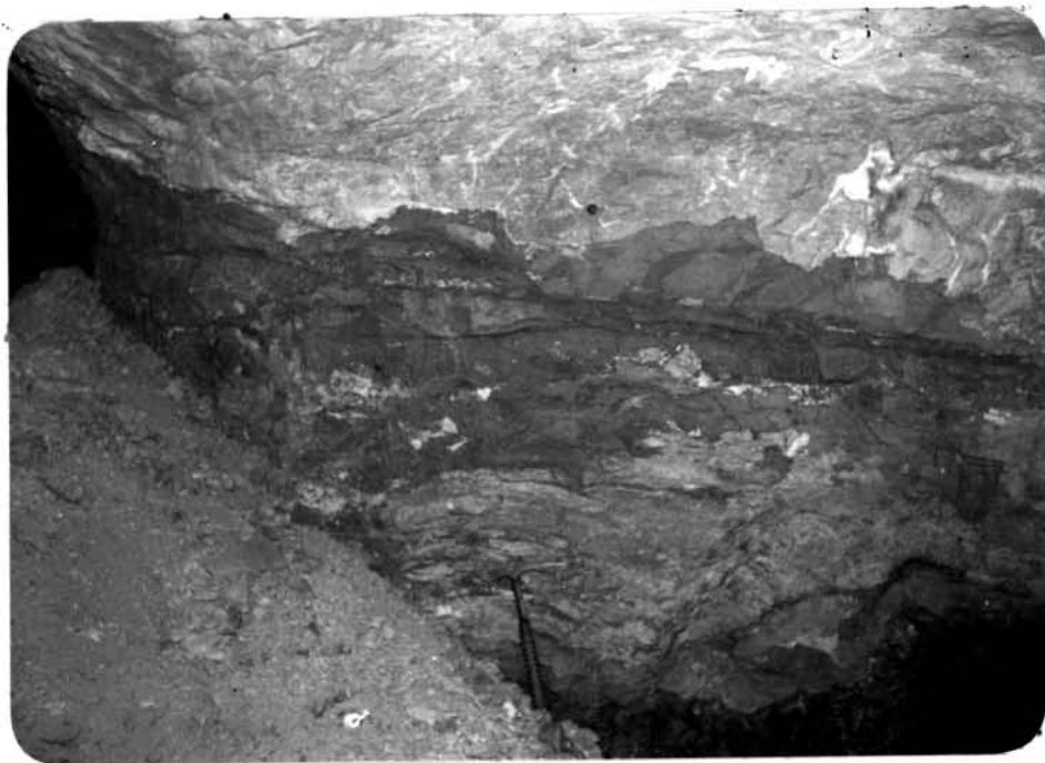
Figure 43 A lens of massive ores showing minor irregularities along the boundary between the sulfide mass and the carbonate host. (Upper ore zone, Song Toh South mine, + 620 m level)
