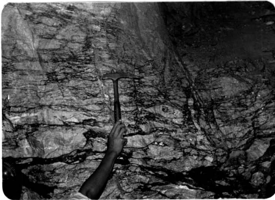
Figure 53 Flaser ores consisted predominantly of lenticular fragments of light gray limestone wrapped by sulfide matrix, showing a perfectly linear structure. (Song Toh South mine, + 640 m level)
