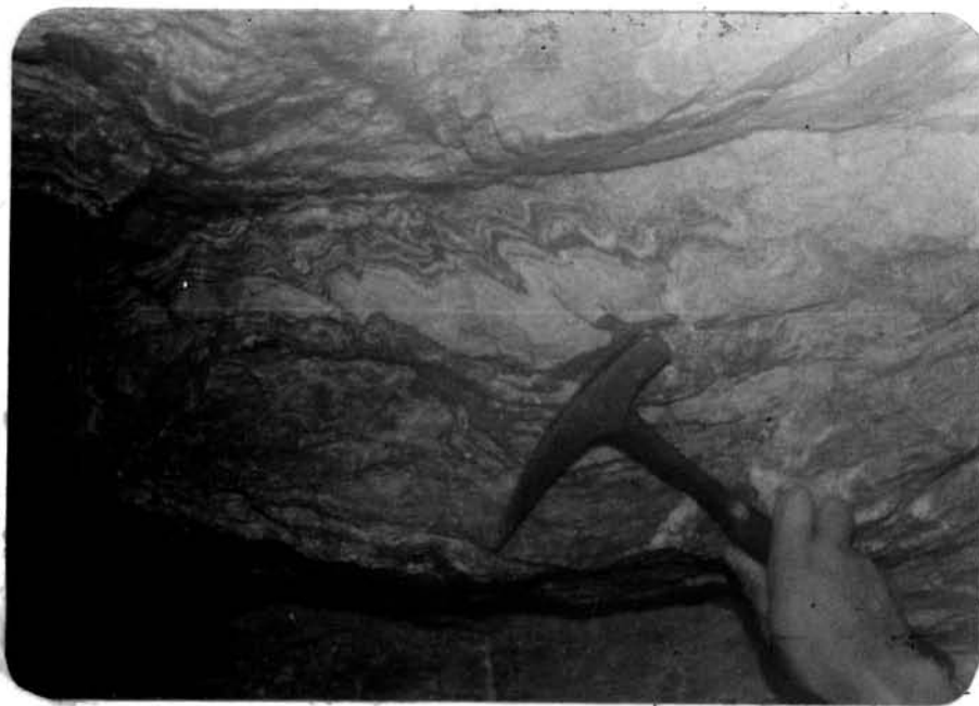
Figure 50 High grade banded ores showing microfolds of their stratified ores probably due to subsequent slumping. (Lower ore zone, Song Toh South mine, + 620 m level)
