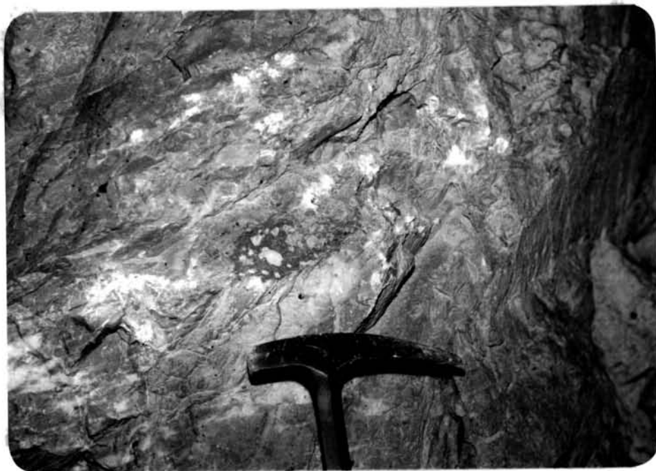
Figure 39 Low grade ore showing a tiny patch of sulfide mass embedded in the limestone host.
