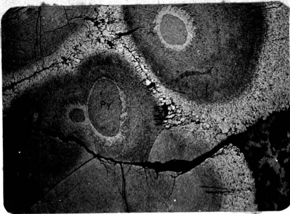
Figure 63 Photomicrograph of colloform pyrite (Py) in the massive ores showing internal zonal growth. (Polished section, 60 x, uncrossed nicols)
