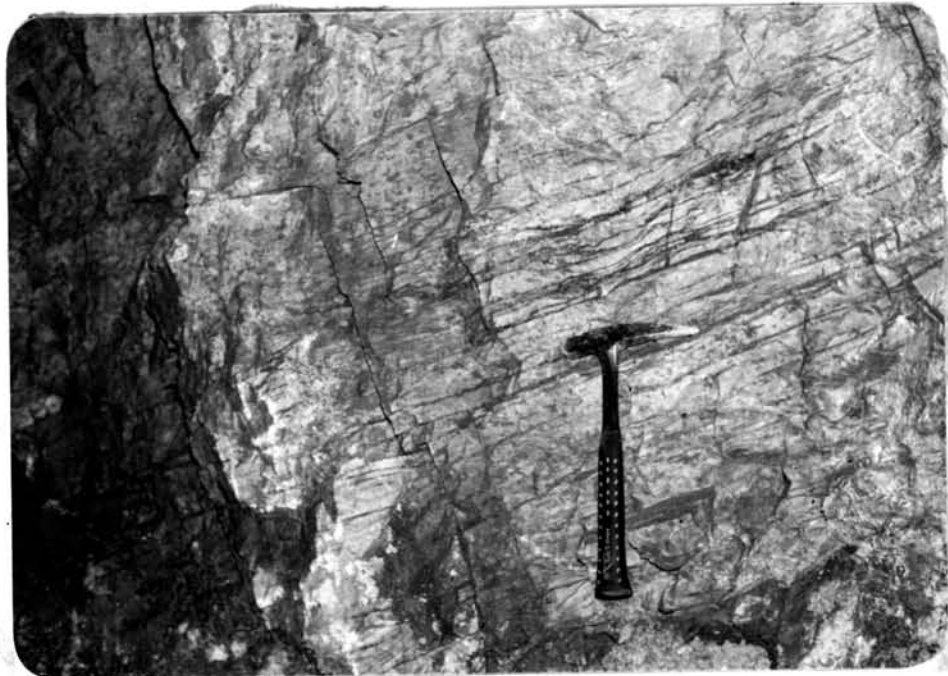
Figure 38 Low grade banded ores showing the concordancies of very thin lenticular sulfide lenses with the bedding of the carbonate host rock.
