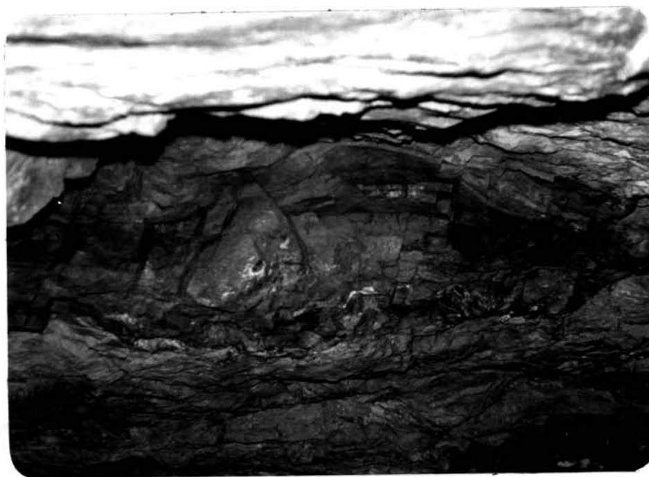
Figure 41 Lenses of massive ores showing sharp, and concordant boundaries with the carbonate host rock. ( A. Song Toh South mine, + 640 m level ; B. upper ore zone, + 620 m level)
