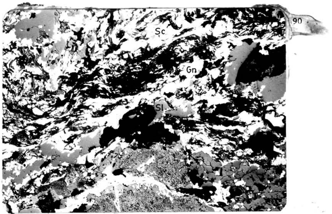
Figure 80 Photomicrograph of banded ores showing ore layering wraps around detached rock fragments. (Polished section, 60 x, uncrossed nicols)
