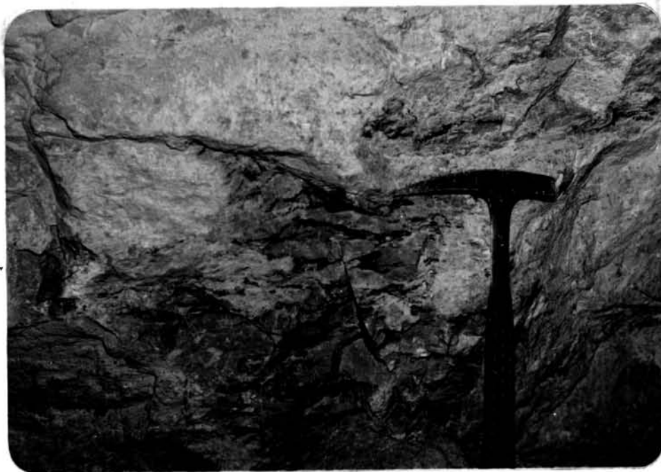
Figure 40 Low grade ore showing the tiny mass of sulfide ores scattered throughout the carbonate host rock. (Upper ore zone, Song Toh South mine, + 620 m level)
