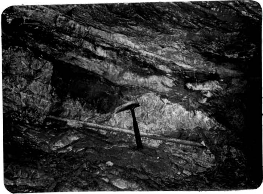
Figure 21 Bedding-plane fault with associated sheared ores. (Song Toh South area, old open-pit mine)
