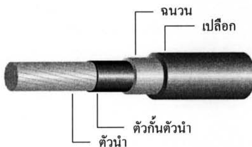
รูปที่ 1.1 Aluminium Space Aerial Power Cables with Cross – Linked Polyethylene Insulated and Sheathed For Rated Voltage 25 kV and 35 kV
