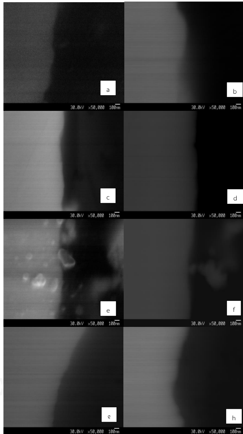
Figure 4.25 SEM images at the interface between zirconia substructure and glass-ceramic liner (x 50000), secondary electron mode in left column and back scattered mode in right column. LG810D (a, b), LLi950D (c, d), VG980D (e,f), VLi850D (g, h)
