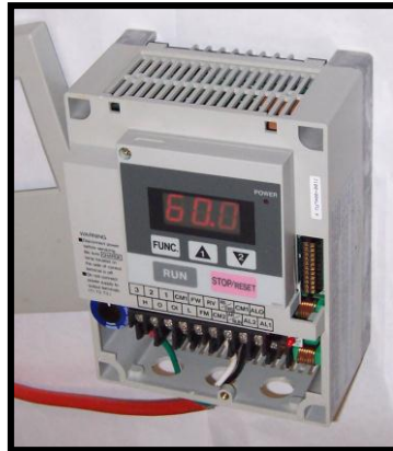
Figure 37 Variable Speed Drive (VSD)
