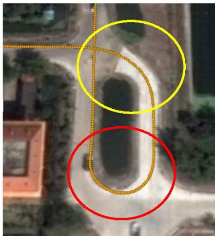
Figure 6 J-turn and U-turn plotted position data
