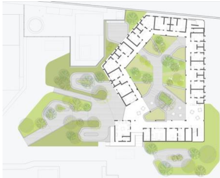
Figure 2.12 The layout of Gheskio hospital emphasizes on the courtyard in maximizing the natural ventilation
