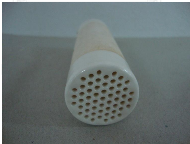
Figure B. 2 Fouled Ceramic Membrane after filtration
