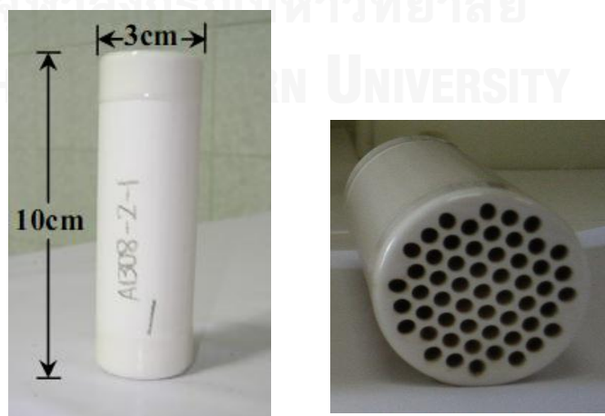
Figure 3. 4 Ceramic membrane modules pore size 0.1 \mu\text{m}
