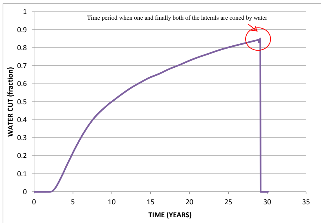
Figure 5.14 Water cut when preset water cut ratio is set at 0.85, of dual-lateral case where L1 is fixed at 20 th grid block with ICV installed
