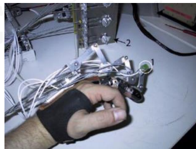
Figure 2.12 A finger exoskeleton developed by A. Wege et al. (picture from A. Wege et al. [16]).
