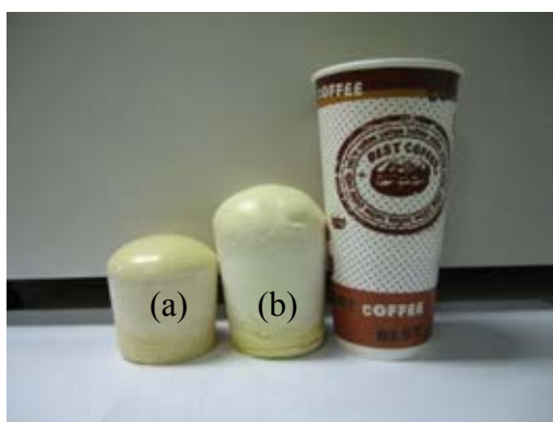
Figure 4.17 The external appearance of RPUR foams prepared at NCO index of 100, 1.0 pbw of water, 2.5 pbw of surfactant, and without adding water: (a) Raypol ® 4218 foams and (b) HBOB foams.
